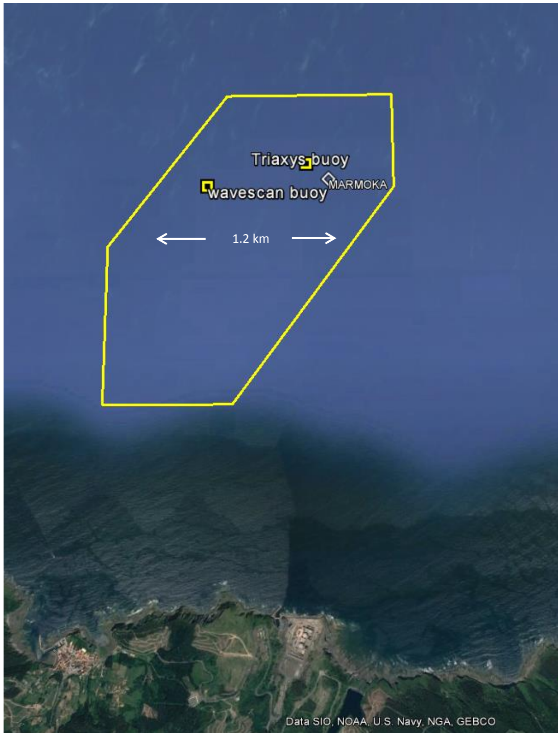
FIGURE 6. POSITION OF OCEANOGRAPHIC BUOYS RELATIVE TO THE WEC (OCEANTEC MARMOK A) AT BIMEP
