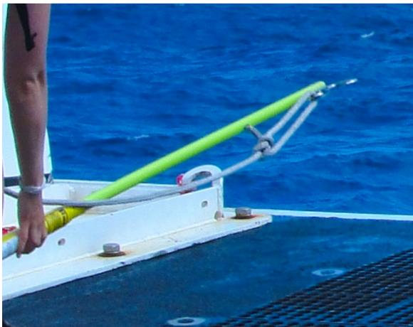
Telescoping fiberglass pole with Wichard mooring hook and line for attaching tag lines to the carousel during recovery.
