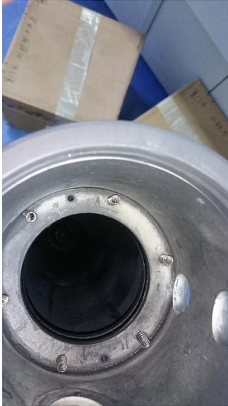
OTE sampling bottle with ball assembly removed to show the stainless steel springs that push up on the floating seal ring (not shown) to seal it against the rotating ball (i.e., the ball in a ball valve).
