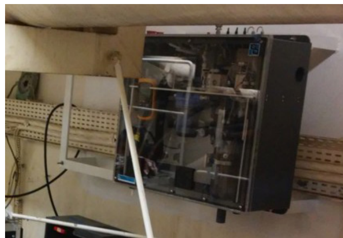
Figure 8. General Oceanics system mounted on a custom built steel frame. As shown in the photo, the wet box is already mounted. The frame extends to the left to the mount of the dry box.
