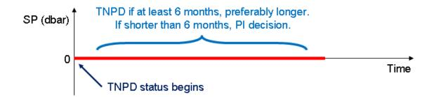
Example (b). There are occasional valid positive SP readings in the first part of the time series, followed by a continuous zero-reading period that does not contain any occasional valid positive readings.
