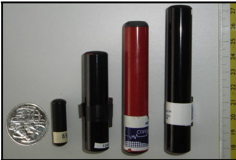
Figure 2. A range of acoustic tags commonly used in CMAR research projects.
