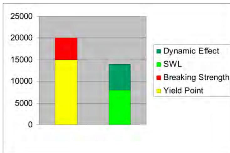
When a tension measuring system is not available which forces using a minimal FS of 5.0, EMT calculations must be done based on mass not weight. In general, the weight of the package, entrained water and the cable or rope in air is roughly equal to the mass. Do not use weight in water for the dynamic loading estimates.
