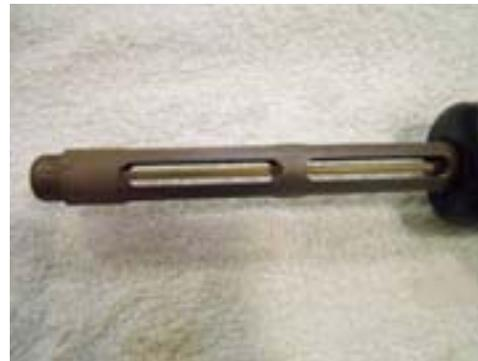
Sensor with the biofouling prevention system after four-week laboratory deployment.
