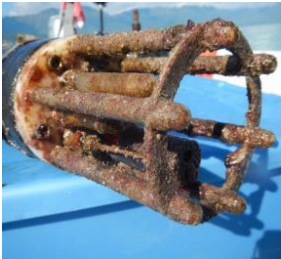
Photo 4. The Idronaut 305 Plus pH sensor prior to and following the 3 month deployment in Kaneohe Bay for the HIMB field test.
