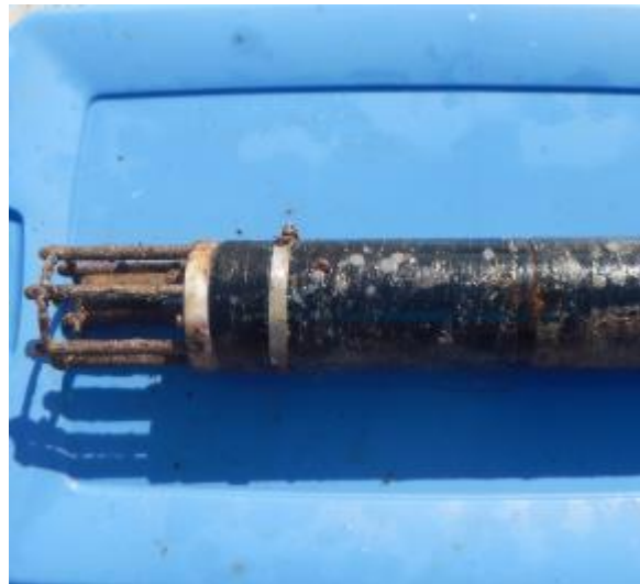
Photo 4. The Idronaut 305 Plus pH sensor prior to and following the 3 month deployment in Kaneohe Bay for the HIMB field test.
