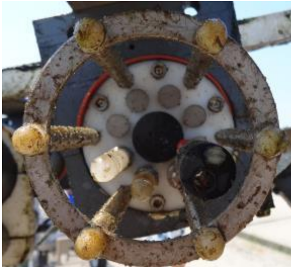
Photo 8. The Idronaut 305 Plus prior to a following 1 month deployment in Lake Michigan for the Great Lakes field test.
