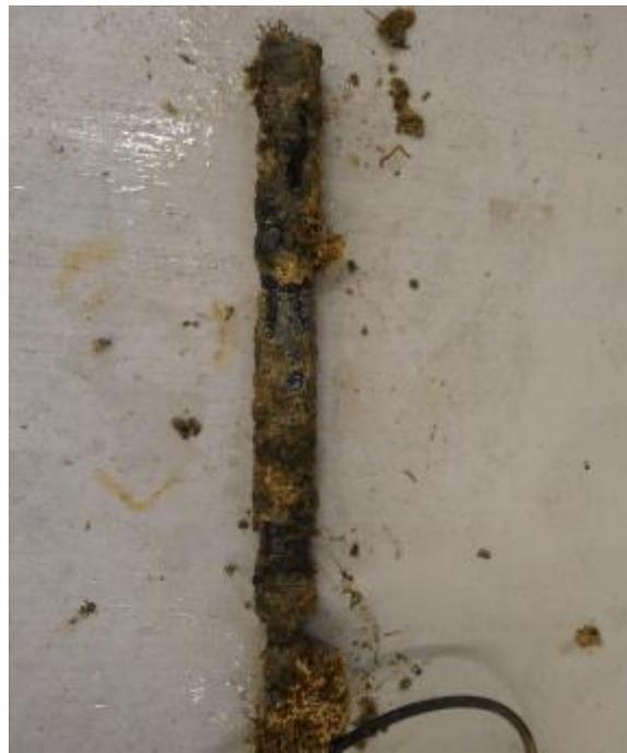
**Photo 3.** The Hach HL4 prior to and following the 18 week CBL field trial.
