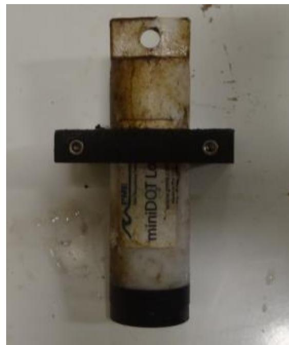
**Photo 2.** PME miniDOT prior to and following 15 week deployment under ice for the MTU field test.
