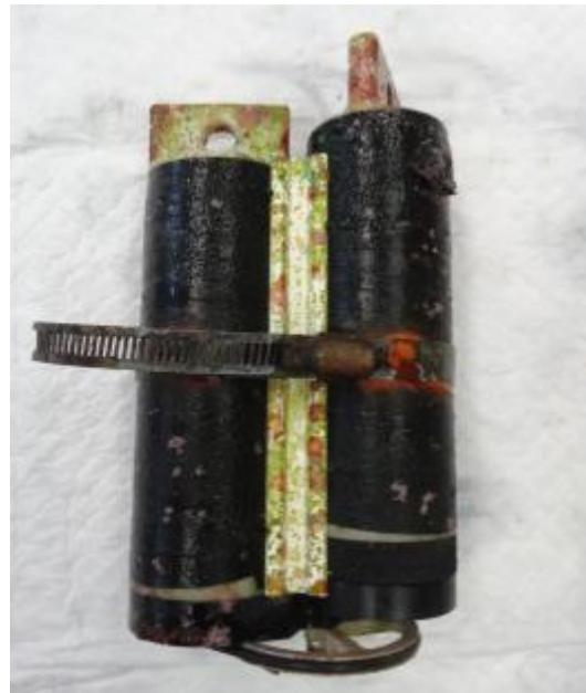
**Photo 6.** The PME miniDOT prior to and following the 18 week HIMB field trial.
