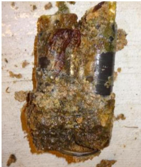
**Photo 4.** The PME miniDOT instrument before and following the 12 week CBL field trial.
