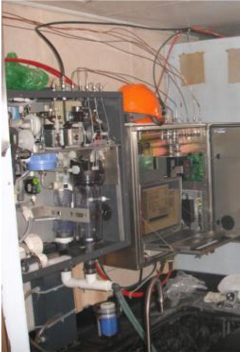
**Figure B.1:** Autonomous underway  $p\text{CO}_2$  system installed on a research ship. The system is built by General Oceanics (<http://www.geraloceanics.com/>) based on specifications resulting from community workshops organized by the International Ocean Carbon Coordination Project (IOCCP). Photo courtesy of Kevin Sullivan, UM/CIMAS.
