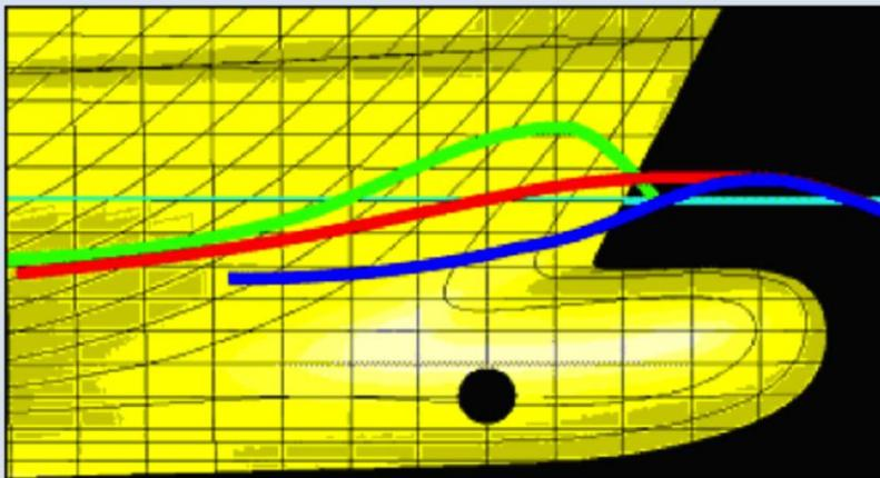
**Figure A.2:** The green line represents schematically the natural bow wave of the hull without the protruding bulb. The blue line represents the wave created by the protruding bulb. The red line is the sum of these two. Notice that the height of the bow wave is substantially reduced, which in turn, reduces the form drag associated with the bow wave. Figure courtesy Jet-Tern Marine.
