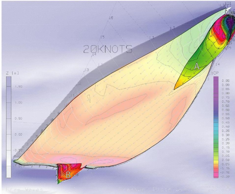
**Figure A.4:** A fish-eye view (distorted proportions) of an ocean-going ferry. The translucent color of the hull sketches the aft-spreading bubble blanket. Only the region around the forward part of the bulbous bow (A) and aft skag (B) remain bubble-free. Remote sensing transducers could be located in either area or in a pod that extends out to the side of the skag (not shown). Figure courtesy Flensburger Schiffbau-Gesellschaft mbH & Co. KG.
