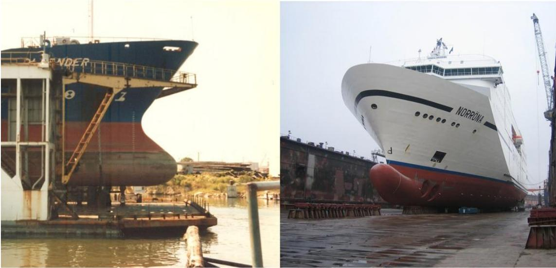
**Figure A.3:** A delta (left) and a nabla (sometimes known as inverted tear drop) bulbous bow (right). Both ships are equipped with ADCPs. The *Oleander* (left) operates between New Jersey and Bermuda, the *Norröna* out of the Faroes to Denmark and Iceland. Photos courtesy T. Rossby.
