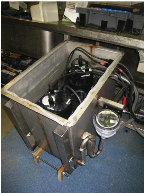
**Figure B.2:** Example of an inline  $p\text{CO}_2$  system produced by Pro-Oceanus. This system is installed in a sealed seachest. Photo courtesy of Brian Ward, Univ. of Galway.
