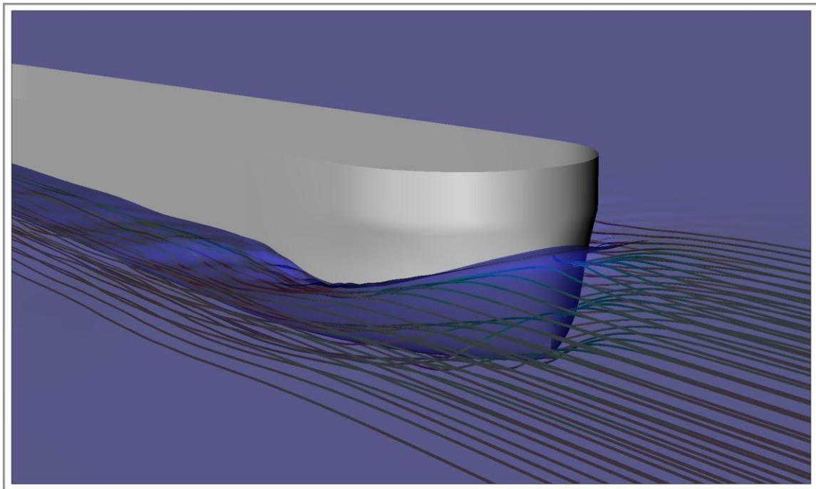
**Figure A.6:** Perspective view of bow wave around a blunt bow bulk carrier. Figure courtesy Deltamarin, Turku, Finland.
