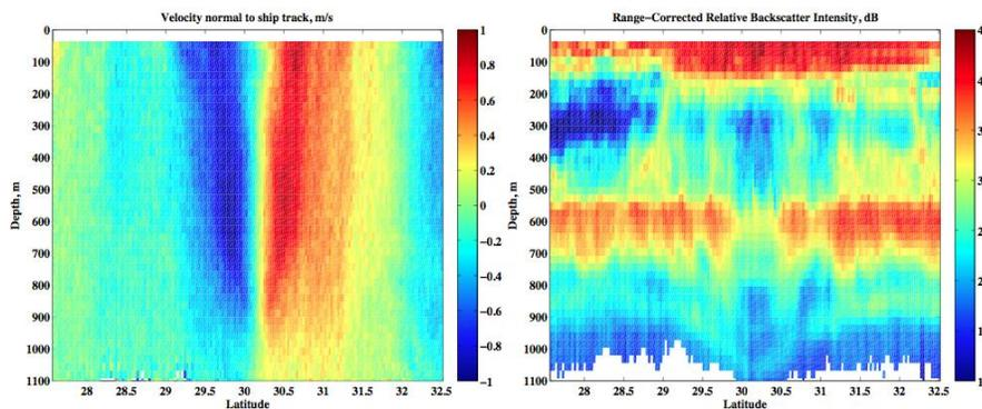
Figure 1.3 ADCP data from the *Explorer of the Seas* transiting an energetic anti-cyclonic eddy at 30°N, 70°W. Velocity normal to the ship track is shown in the left panel and backscatter signal strength is shown in the right panel. Note the interruption of deep scattering layer at 600 m and the deepening of a second scattering layer at 900m (Rossby et al., 2011). Used with permission of the American Geophysical Union.
