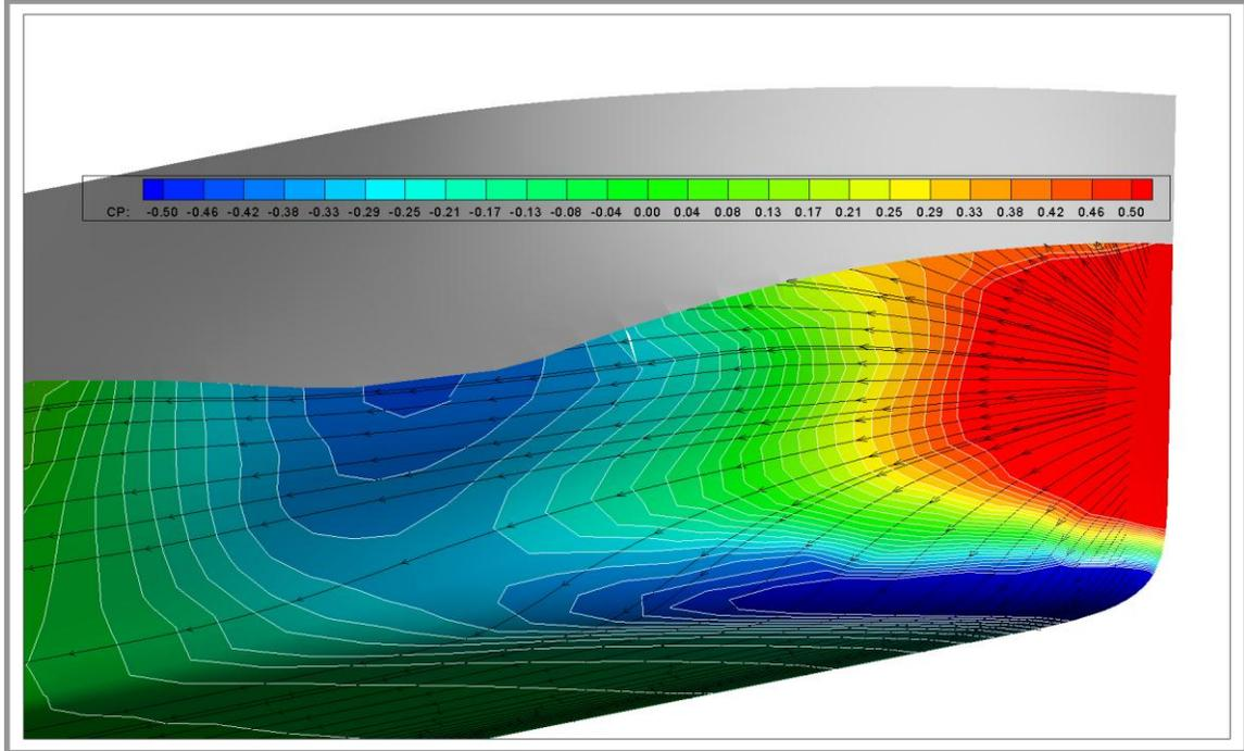
**Figure A.5:** CFD study of flow around the bow of a bulk carrier. One sees how the bow waves wets the side of the vessel and the relatively horizontal pattern to the streamlines. The color indicates pressure (red = high static pressure, blue = high dynamic pressure). Figure courtesy of Deltamarin, Turku, Finland.
