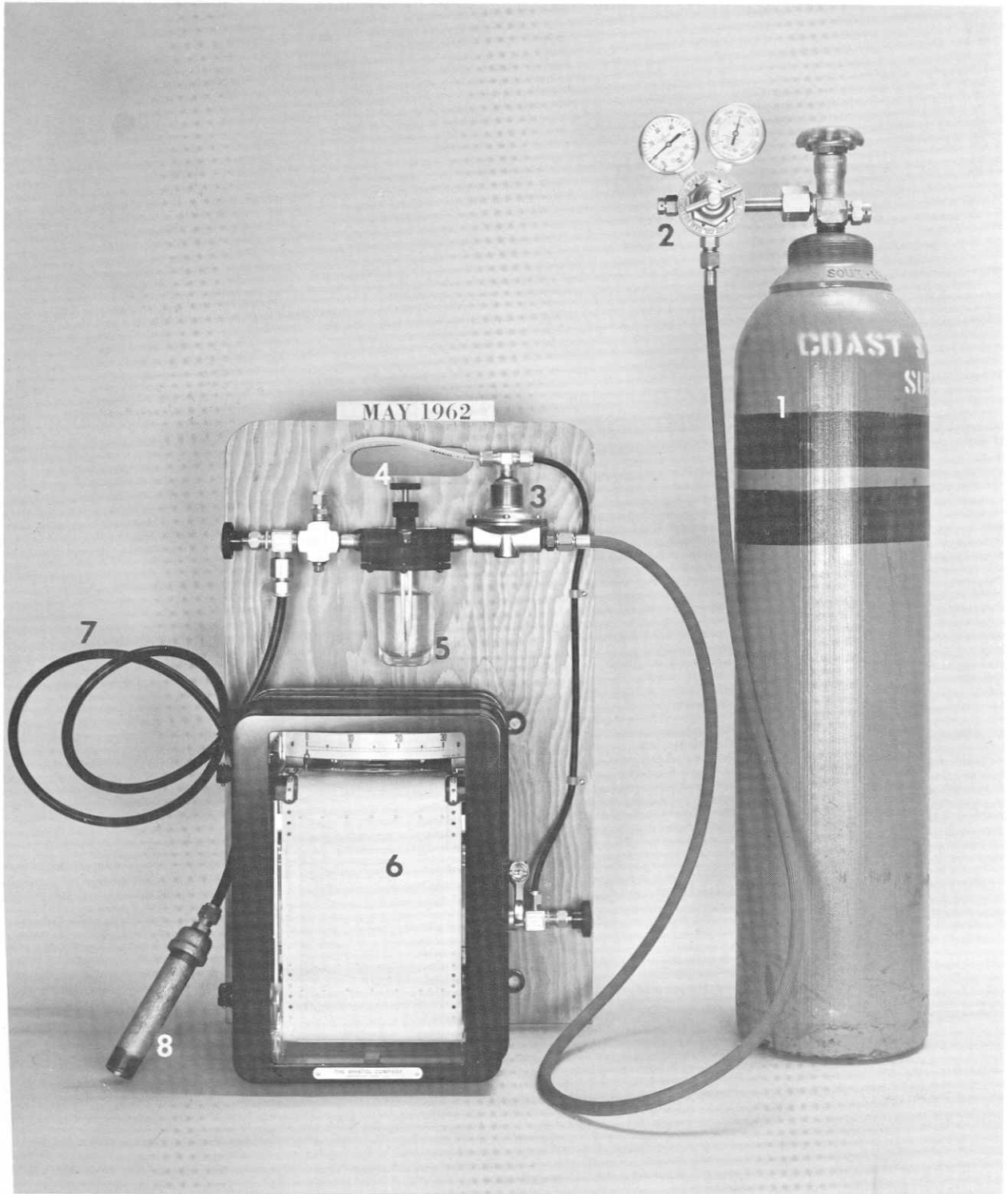
FIGURE 4.—Gas-purging pressure tide gage.
