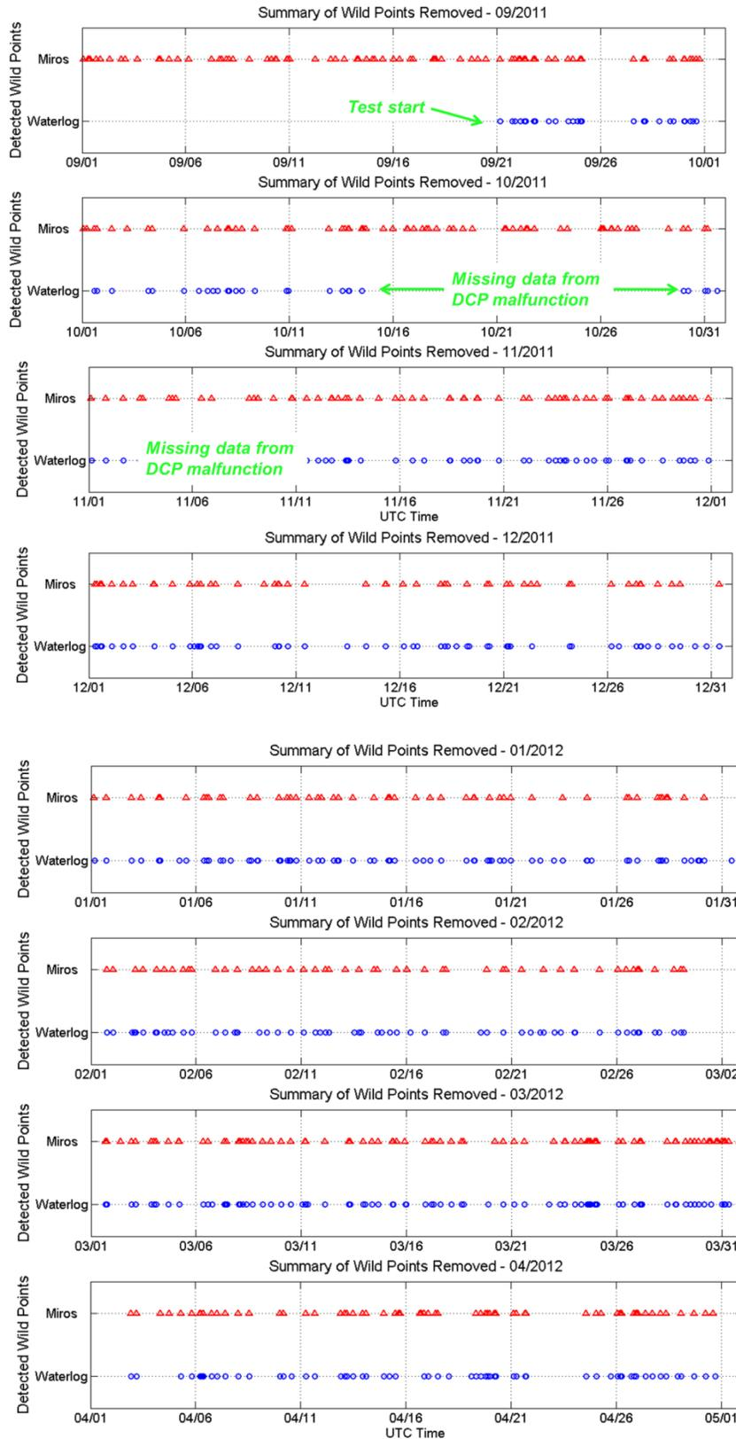
Figure 26. Time and number of wild points detected and removed from both sensors' records.
