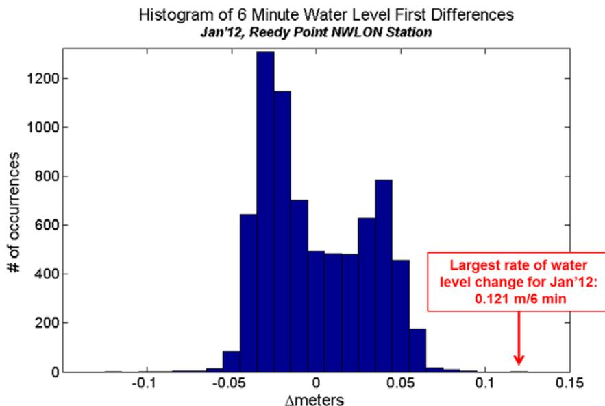
**Figure 24.** Sample histogram of 6-min water level first difference generated from January 2012 water level record at Point, DE NWLON station.
