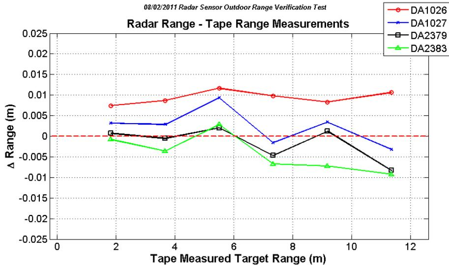
Figure 9. Results from range accuracy verification test.
