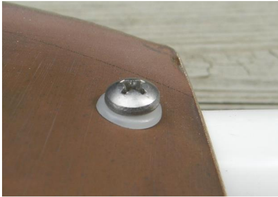
Figure 2 - Nylon washers isolated the dissimilar metals of the stainless steel screws and the test plates
