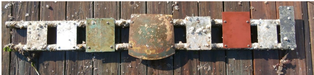
Figure 4 - The eight plates are shown after uniformly cleaning each with a directed jet of water.
