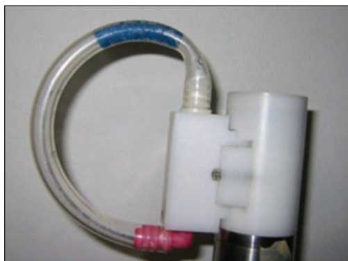
Figure 13. Tygon tubing with damp sponge looped around inlet and exhaust of SBE 43 sensor for storage
