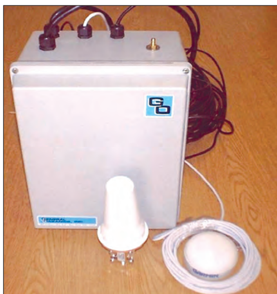
Figure 3: Satellite deck box w/ GPS & Iridium Antenna
