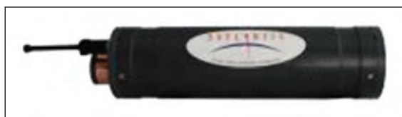
Figure 10. Satlantic SeaFET Ocean pH Sensor
