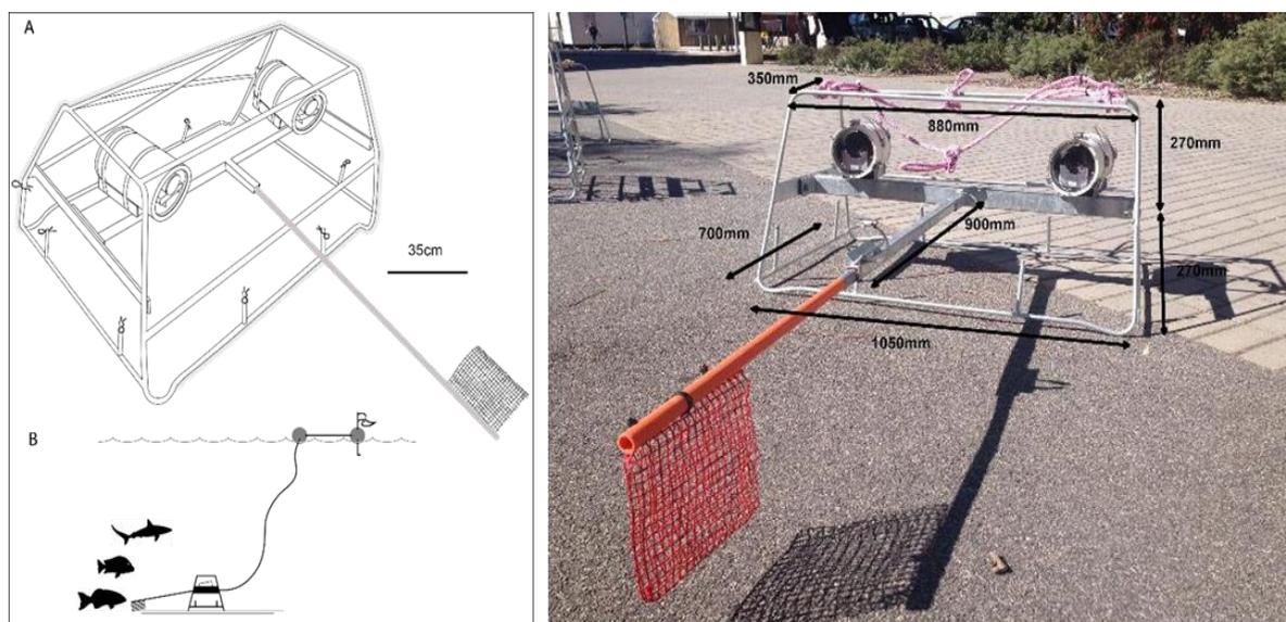
Figure 5.1 Left A: typical stereo baited remote underwater video (stereo-BRUV) and Left B: schematic of typical deployment setup of a stereo-BRUV unit sitting upright on the substrata with a rope leading to two buoys on the surface (Source: T. Simmonds/AIMS). Right: A photograph of a typical stereo-BRUV with the dimensions of the frame.
