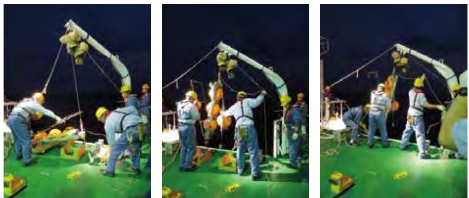
Fig.10 Launch operations using a davit (Left and center: hoisting the Edokko Mark I, Right: swinging it out of the ship)
