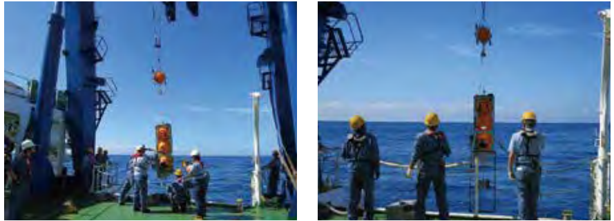
Fig.11 Launch operation using an A frame
