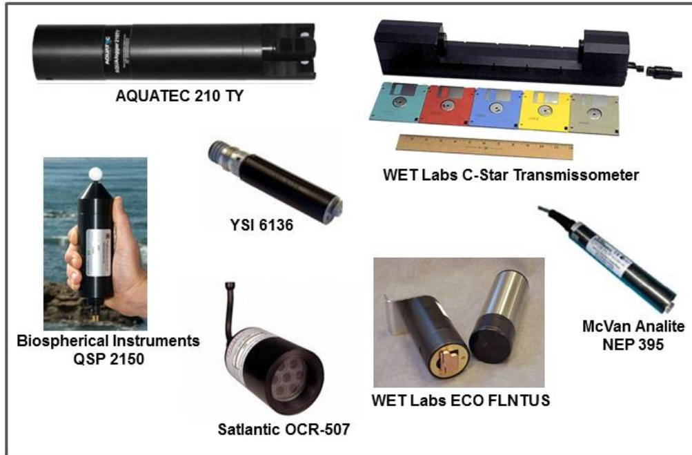
Figure 2-1. Examples of widely used ocean optics sensors.
