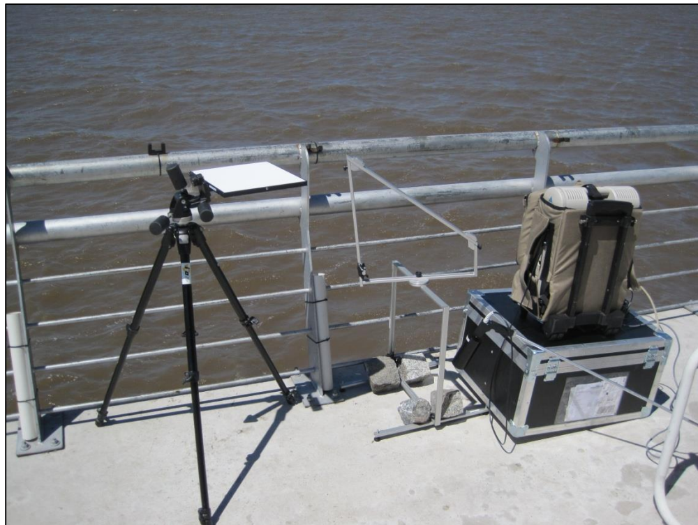
Figure 2-2. Shows the shipboard deployment of an ASD FieldSpec FR (right) and Spectralon plaque (left) used for observations of above-water radiance. The pistol grip and lens limit the field of view to one degree. (Photo courtesy of Dr. Ana Dogliotti/CONICET/UBA)
