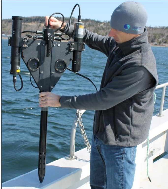
Figure 2-5. A variety of optical instruments (including multi-spectral downwelling irradiance and upwelling radiance) are installed and deployed aboard this Satlantic Profiler II, which can free-fall through the water column or be lowered using a tether. (Photo courtesy of Todd Yeadon/Sea-Bird Scientific)
