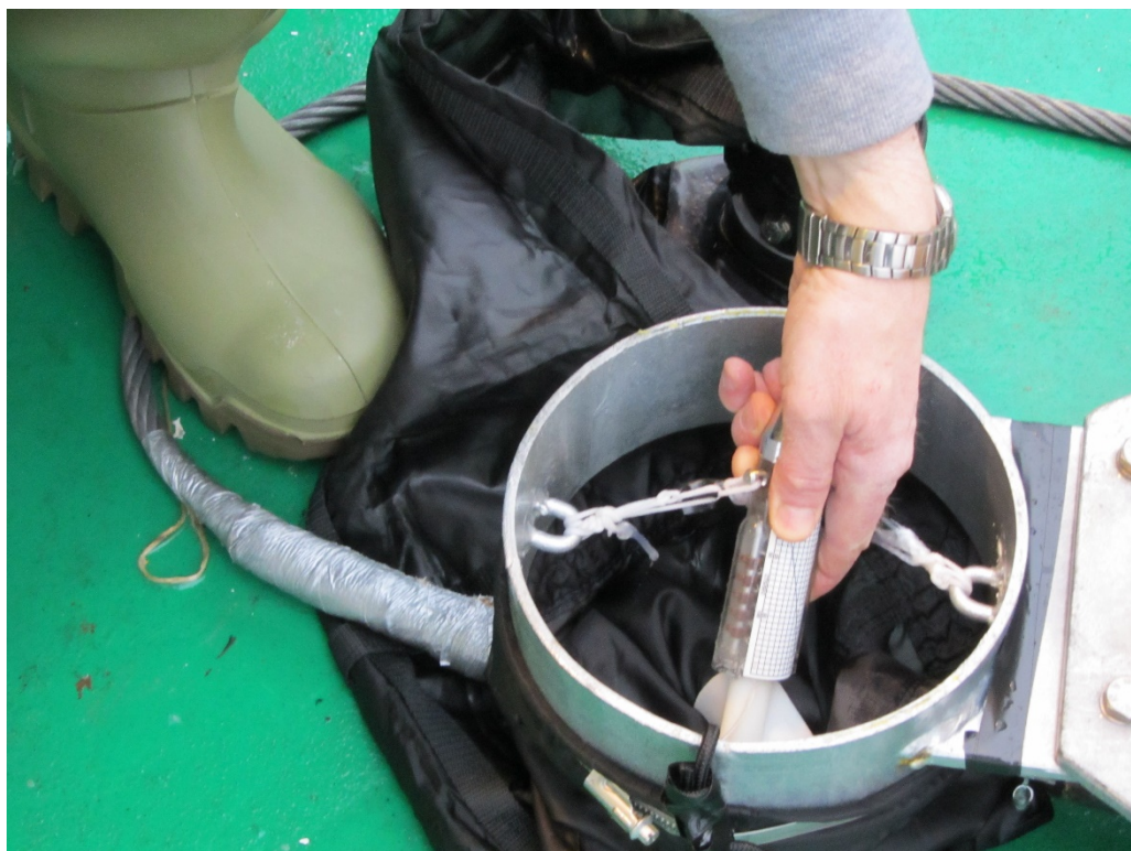
Flowmeter attachment inside MIKeyM ring
