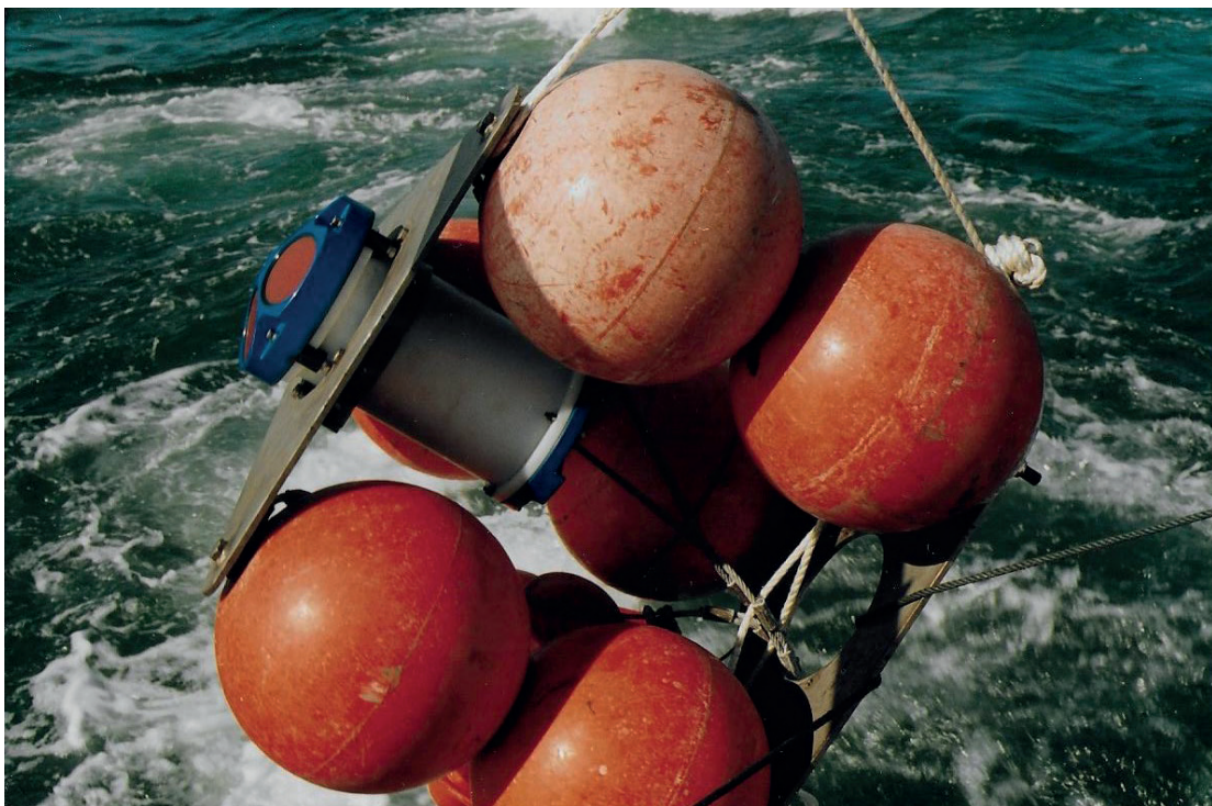
Figure 9: An ADCP in short mooring flotation collar designed for low current environment (© 2021 Blue Ocean Consulting Ltd)
