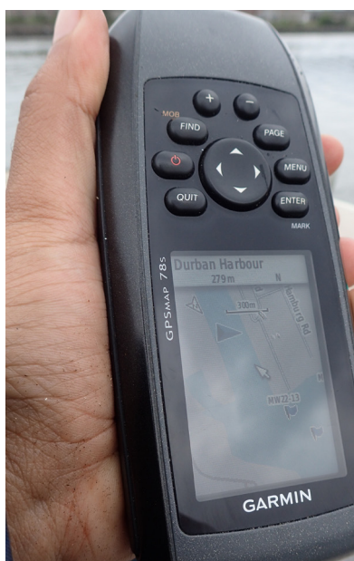
Figure 6: An example of a field map showing the positions where sediment is to be sampled. The vessel skipper should ideally have a separate sheet showing the order in which the sites should be sampled. In this case, the sediment at Sites A1, A2, and A3 was known from previous surveys to be the most contaminated and was sampled last to limit the possibility of contaminant transfer amongst samples.
