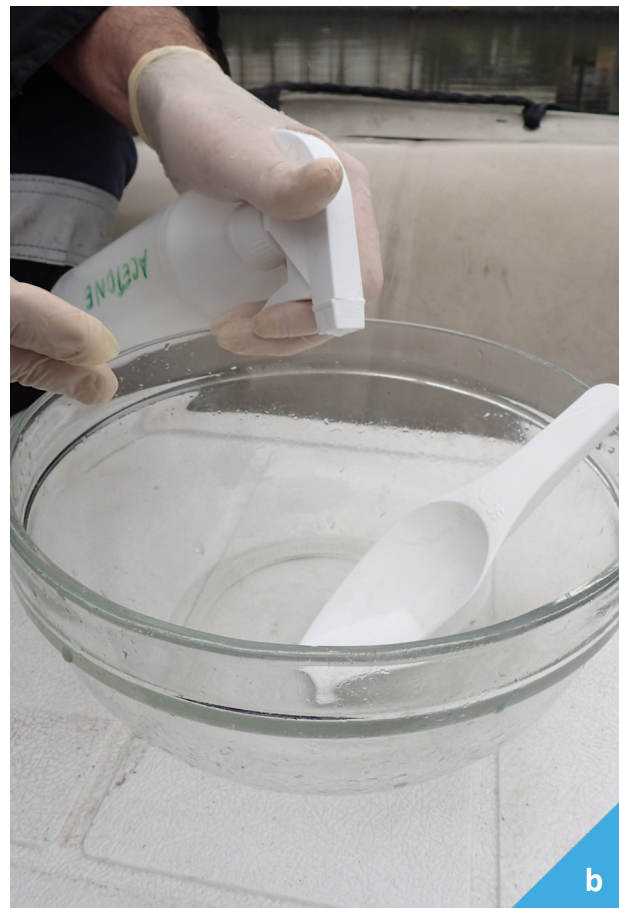
Figure 22: a) Transferred sediment samples in the appropriate sample containers for specific analyses. b) Spraying the mixing bowl with acetone before transferring the next sediment sample into it.
