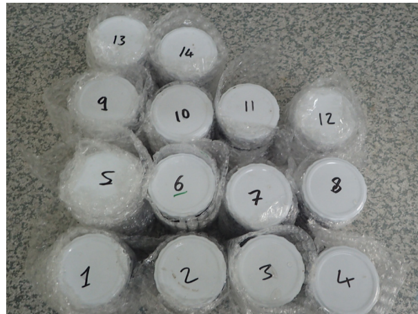
Figure 24: Samples should be reconciled in the laboratory with the Sampling and Analysis Plan and field sample log and data sheets and then transferred to a fridge or freezer. Note the site codes on the lids of the containers. The site code and additional information were also included on sample labels affixed to the sides of the containers.
