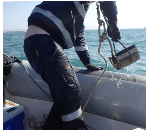
Figure 15: The petite Ponar grab is small enough to be operated by hand. Note the top flap and screen that can be removed to allow access to surface sediment in the grab to obtain your sample.
