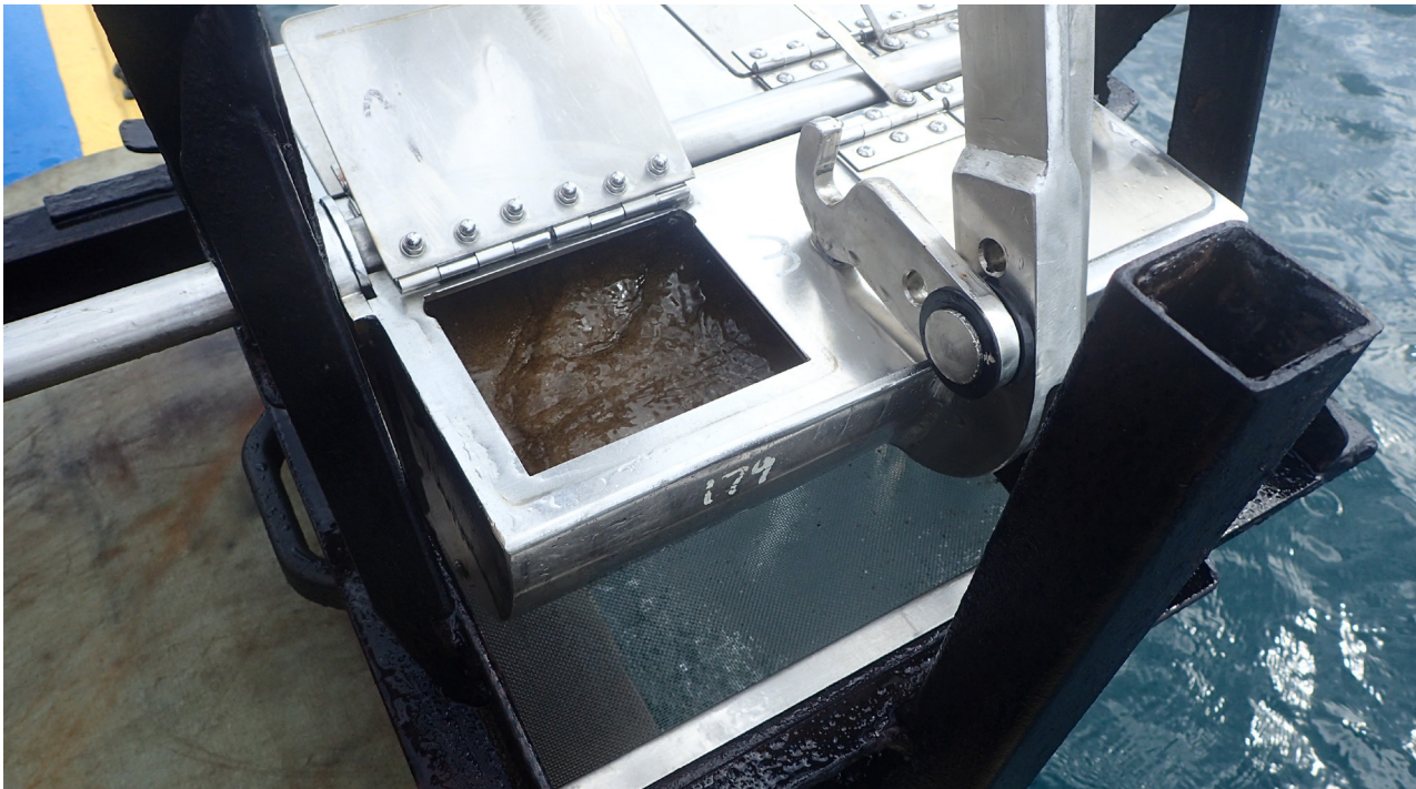
Figure 17: A retrieved grab sampler showing water overlying sediment in the grab. The presence of clear water overlying sediment in the grab sampler is one of the criteria used to accept a sediment sample for processing. The water must be siphoned off using a tube before sediment is removed from the grab.
