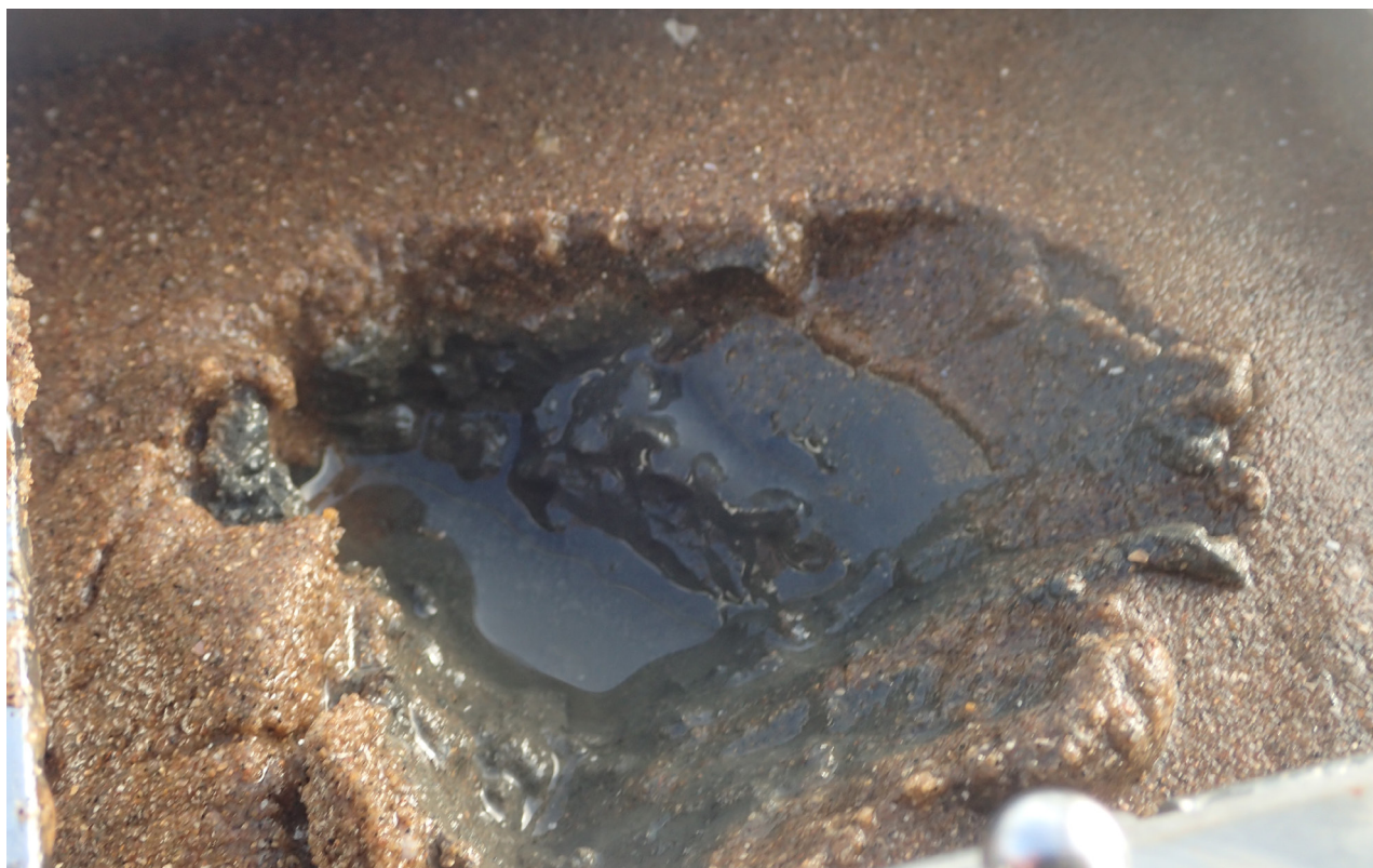
Figure 20: Sediment for analysis is usually removed from the top few centimetres of sediment in a grab. In this case, a scoop was used to remove the required volume of sediment from each quadrant of the grab (specific to the grab in this photo), and the volumes were then combined to provide sufficient sediment for analysis.
