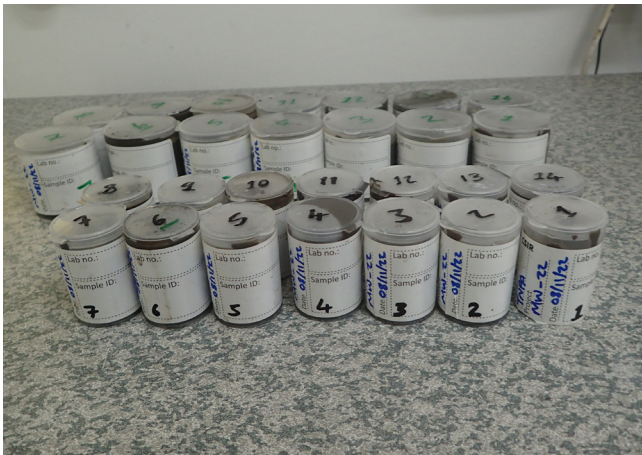
Figure 24: Samples should be reconciled in the laboratory with the Sampling and Analysis Plan and field sample log and data sheets and then transferred to a fridge or freezer. Note the site codes on the lids of the containers. The site code and additional information were also included on sample labels affixed to the sides of the containers.
