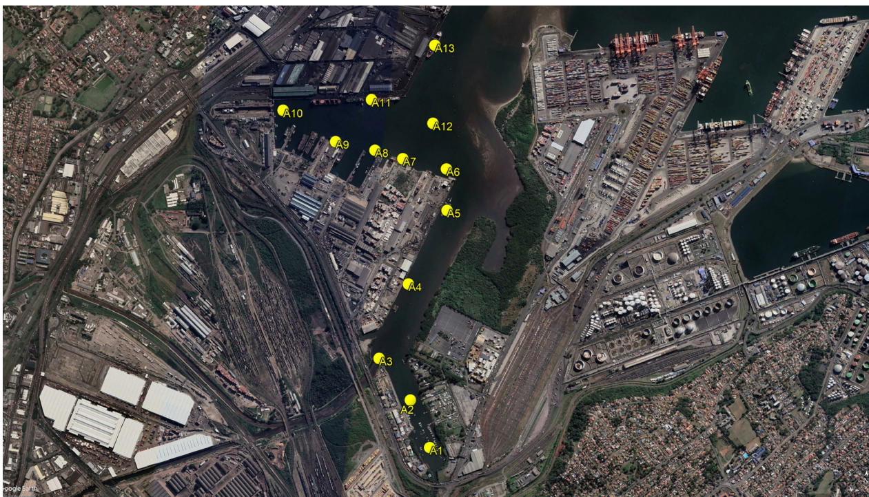
Figure 6: An example of a field map showing the positions where sediment is to be sampled. The vessel skipper should ideally have a separate sheet showing the order in which the sites should be sampled. In this case, the sediment at Sites A1, A2, and A3 was known from previous surveys to be the most contaminated and was sampled last to limit the possibility of contaminant transfer amongst samples.
