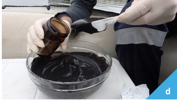
Figure 21: After transferring sediment to a mixing bowl (a) the sediment must be vigorously homogenised until it has a consistent colour and texture (b and c). The sediment can then be transferred to sample storage containers (d). Note in this example the grab does not have top flaps and the entire contents were thus emptied into the glass bowl.
