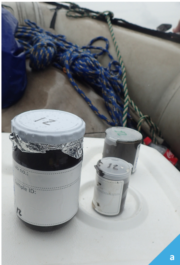
Figure 22: a) Transferred sediment samples in the appropriate sample containers for specific analyses. b) Spraying the mixing bowl with acetone before transferring the next sediment sample into it.
