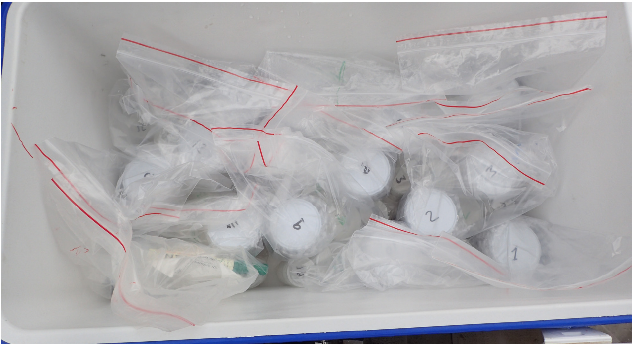
Figure 23: Samples should be stored in a cooler box in the field. In this case, the samples for each site are stored in separate bags. Note that the ice bricks have been removed from the cooler box for display purposes.
