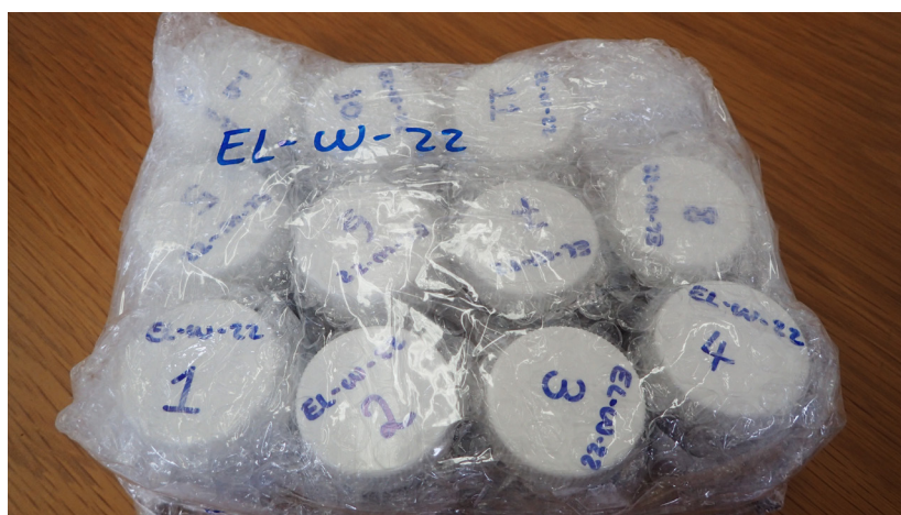
Figure 26: Sample storage containers should be wrapped in bubble wrap to prevent damage while they are being shipped to the recipient analytical laboratory. The sediment samples in this example were freeze dried and ball milled before shipping. Note the site codes on the lids of the containers. The site code and additional information was also included on sample labels affixed to the sides of the containers.
