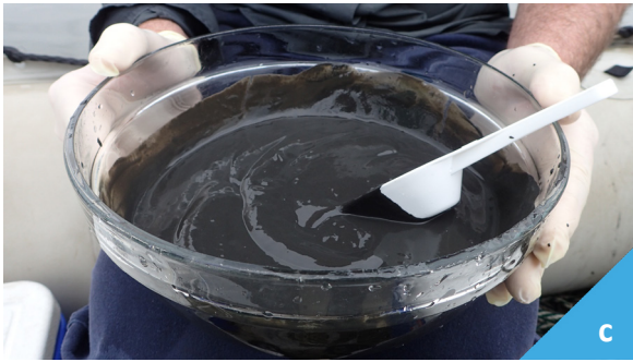
Figure 21: After transferring sediment to a mixing bowl (a) the sediment must be vigorously homogenised until it has a consistent colour and texture (b and c). The sediment can then be transferred to sample storage containers (d). Note in this example the grab does not have top flaps and the entire contents were thus emptied into the glass bowl.
