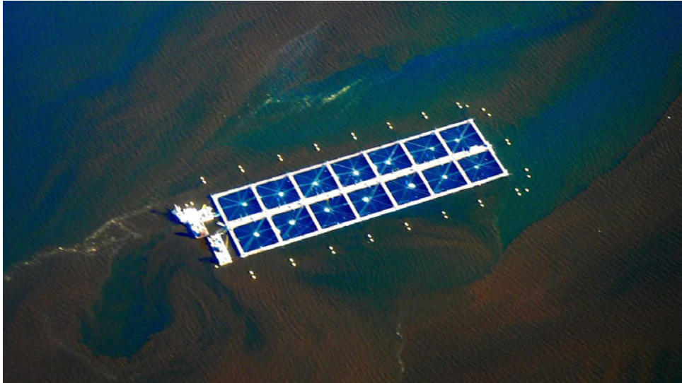
Figure 9.2. Aerial photograph of net pens with airlift upwelling during a Heterosigma bloom in British Columbia showing dramatic colour difference in inside pens versus outside pens. Photo courtesy of Cermaq Canada Ltd. as published in Sellner and Rensel (2018).
