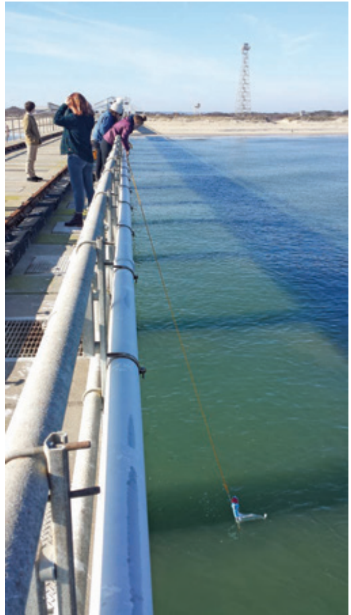
Figure 2. Bagel has a breached net and bottle, which calls for a restart of the tow. Students must repeatedly dunk the frame until it is submerged properly, a frustrating exercise that potentially compromises the sample even during relatively good conditions.
