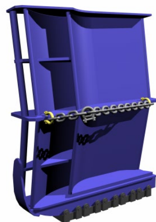
Fig 3.9 Modern multi foil door
