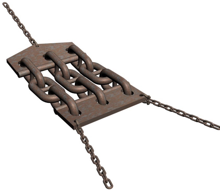
Fig 5.4 Chain clump weight
