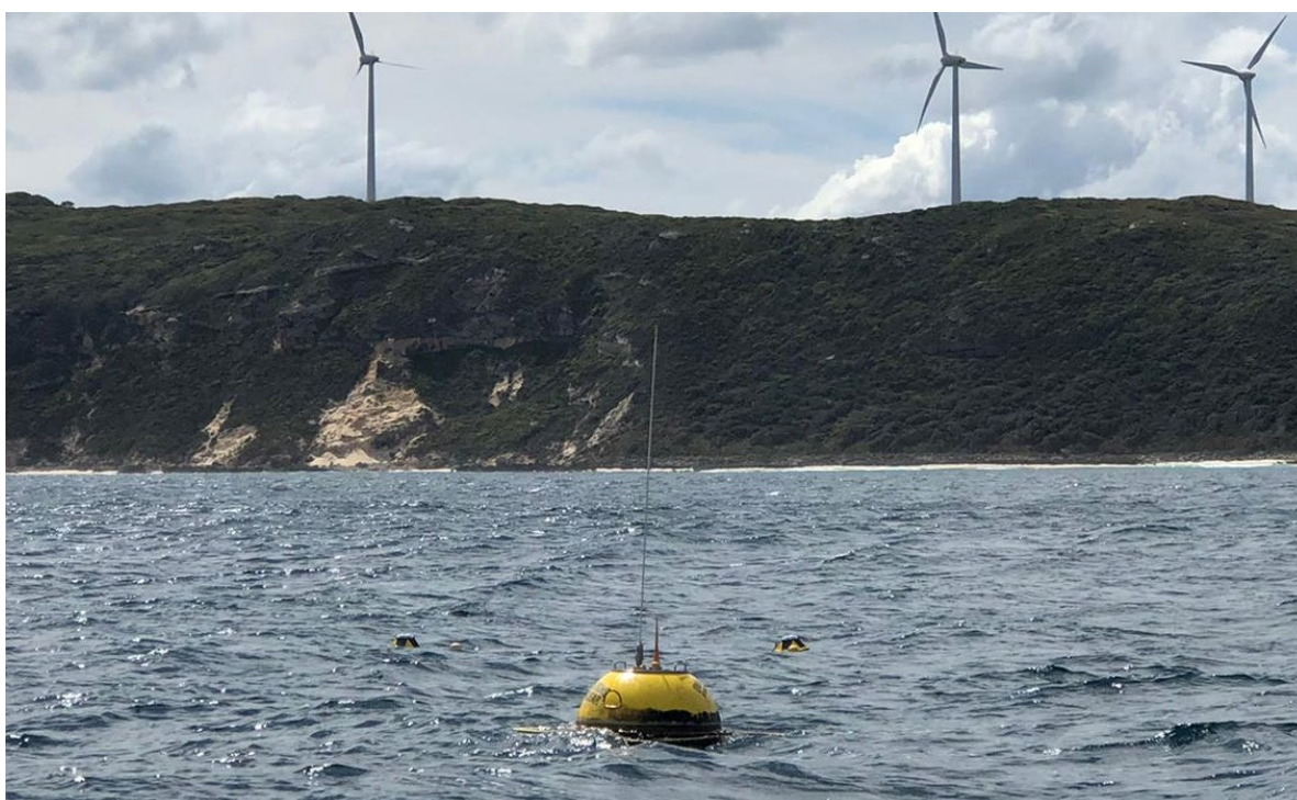
Figure 1. Large and small format wave buoys deployed at Torbay near Albany, Western Australia - a Datawell DWR4 (0.9 m diameter) in the foreground with two Sofar Spotter buoys (0.4 m diameter) in the background. (source: J. Hansen)
