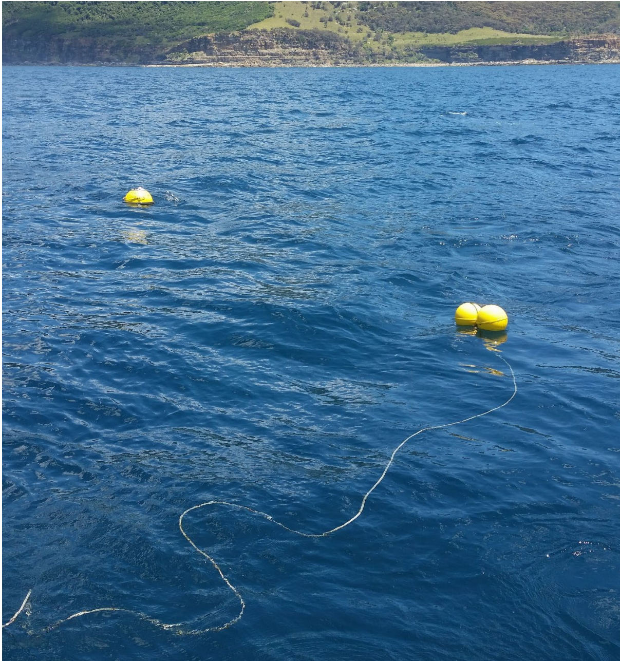
Figure 9. When deploying a wave buoy mooring, the wave buoy should be placed in the water first, then the mooring line (including surface floats if present) laid out steadily as the vessel approaches the deployment location (taking care not to tow the wave buoy), and the anchor weight deployed last. Compare the equipment in the water here with that shown on deck in Figure 5 (source: M Kinsela)
