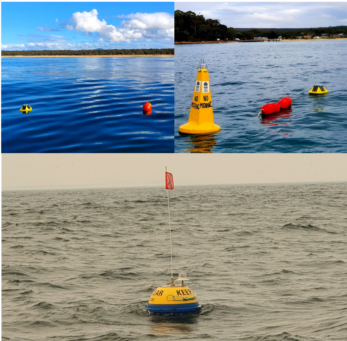
Figure 8. Sofar Spotter wave buoys deployed on shallow-water nearshore moorings with different levels of visibility: the basic swing mooring (top left) is located in a low-traffic setting and is less visible, while the high-visibility swing mooring (top right) is located in a high-traffic setting – note the spar buoy (special marker) with light and surface line floats to increase visibility. For deep-water buoy deployments without surface floats a flag can increase visibility of the wave buoy (bottom). (source: M. Kinsela)
