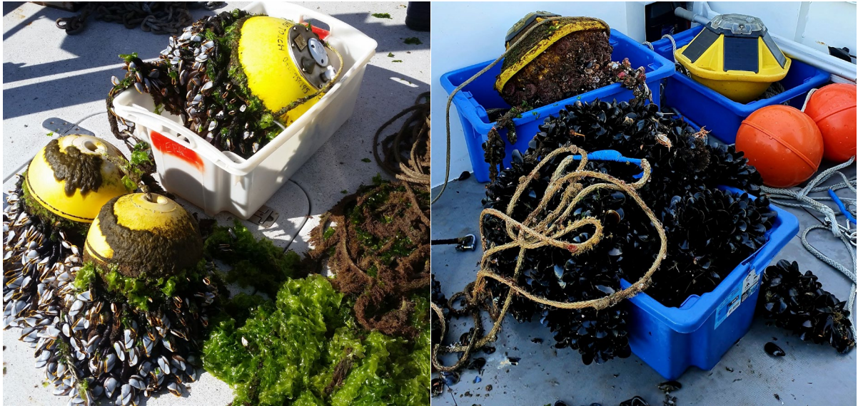
Figure 10. Examples of a heavy fouling of wave buoys and moorings with goose barnacles ( Lepas pectinata ) and green algae ( Ulva sp. ) (left), and blue mussels ( Mytilus galloprovincialis ) (right). (source: M. Kinsela)
