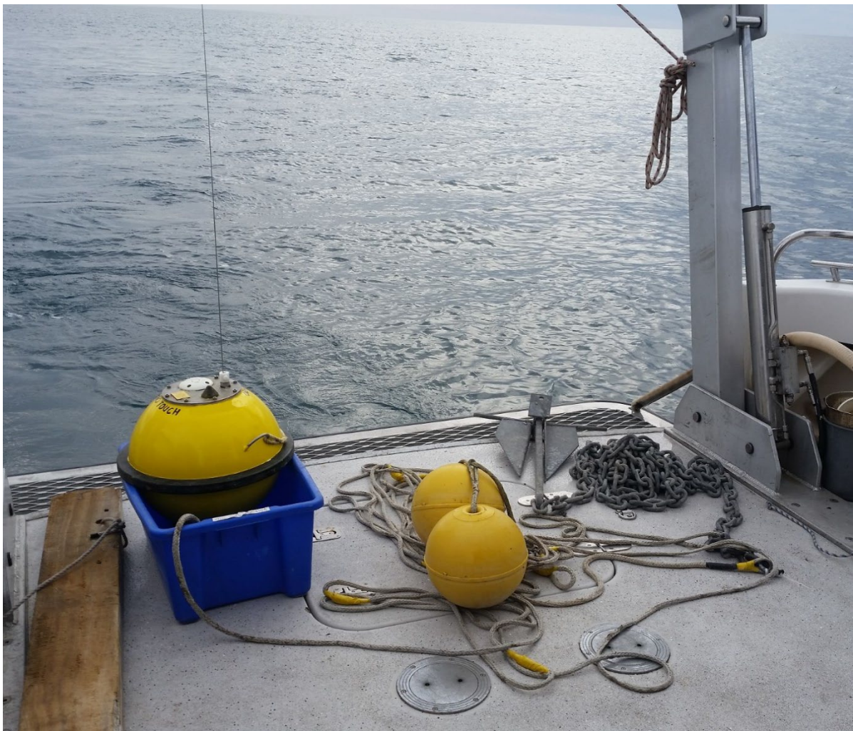
Figure 5. Components of a shallow-water wave buoy mooring for a small format Datawell DWR-G4 buoy laid out on deck for deployment, including: wave buoy, surface floats, mooring line with in-line weights, chain weight and anchor. The mooring design is similar to the example diagram shown in Figure 7 . (source. M. Kinsela)
