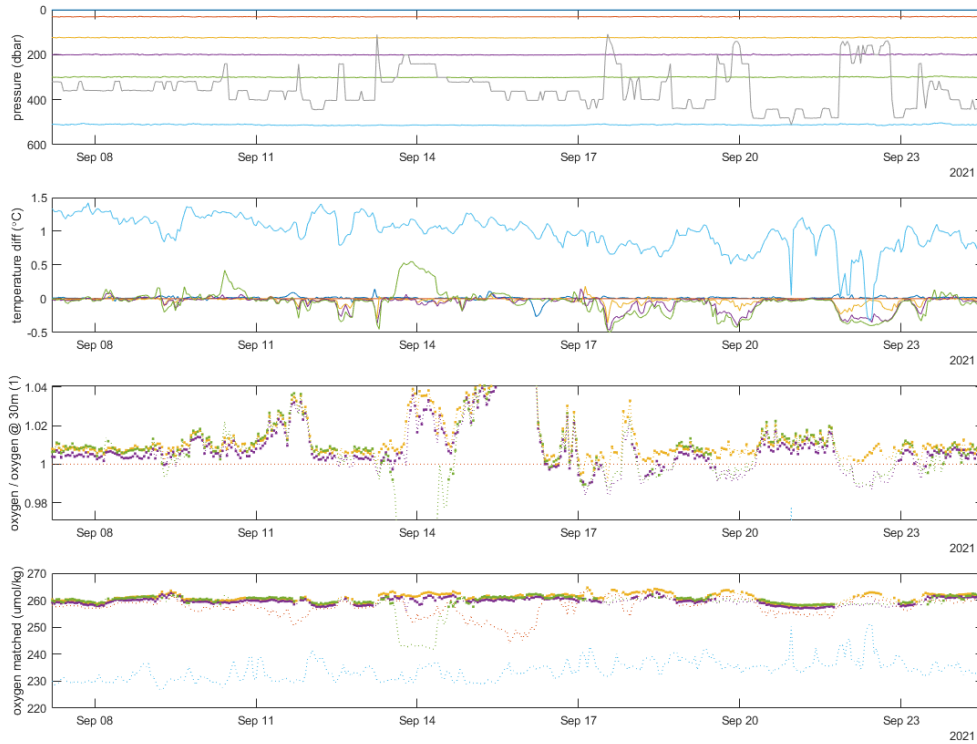
Figure 19 zoom of September where mix layer is > 400m, 30m sensor can read low even when the temperature are the same and sensors are within the mix layer depth.
