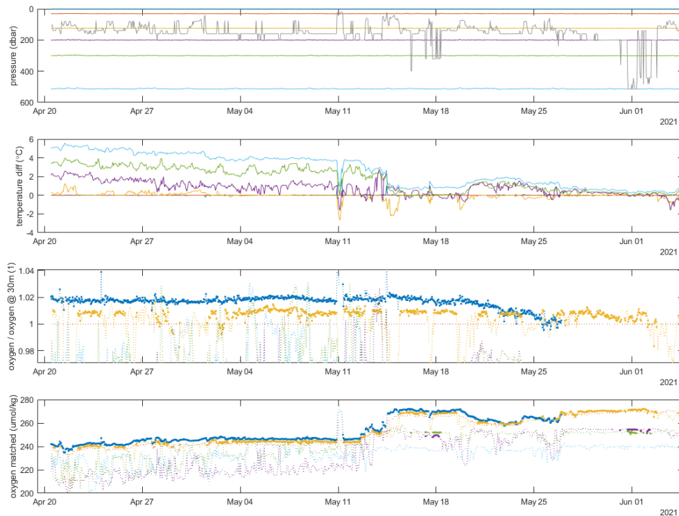
Figure 18 Initial comparison, Optode 2% high compared to 30m sensor, 125m sensor is ~1%
