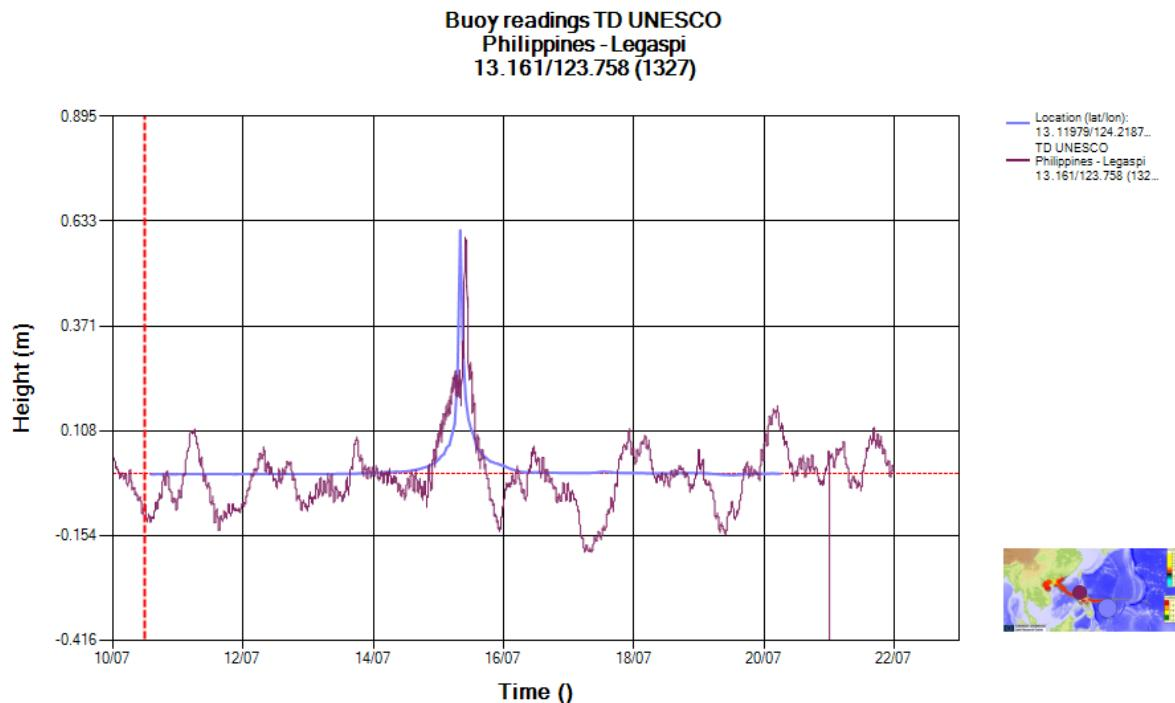
**Figure 1** - Comparison of measured and calculated storm surge in Philippines, during the Tropical Cyclone RAMASSUN (July 2014)
