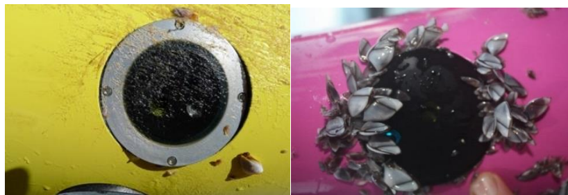
Figure 13 Examples of biofouling growing on the windows of optical sensors in a (left) Slocum glider and (right) Seaglider.
