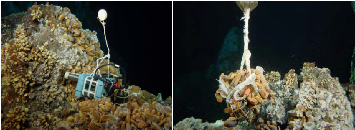
Fig. 11 Aanderaa oxygen sensor, equipped with the electrolysis antifouling system. A) Deployment “Exomar” 2005. B) recovering “Momareto” 2006. (Photos, courtesy of Ifremer)
