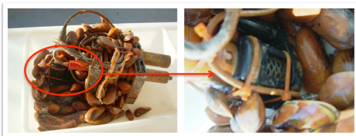
Fig. 12 A) Global view of macro fouling after 12 months. B) Detailed view of local protection efficiency. (Photos, courtesy of Ifremer)
