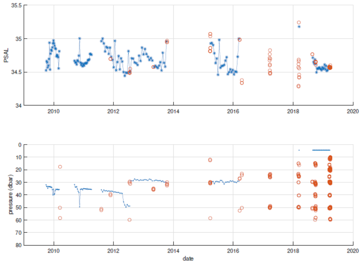
Figure 3. Multi-year comparison of RAS and Shipboard CTD bottles (open circles) a. salinities and b. depths of sampling
