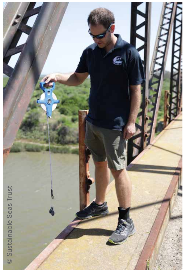
Figure 4: A weighted measuring tape is used to measure water depth from a bridge in Gqeberha, South Africa.
