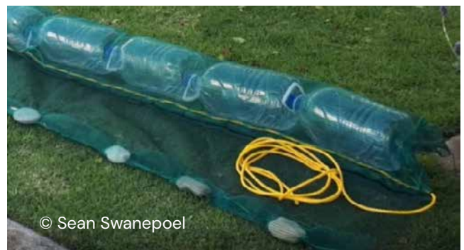
Figure 6: A plastic bottle boom with a mesh curtain weighed down by rocks.
