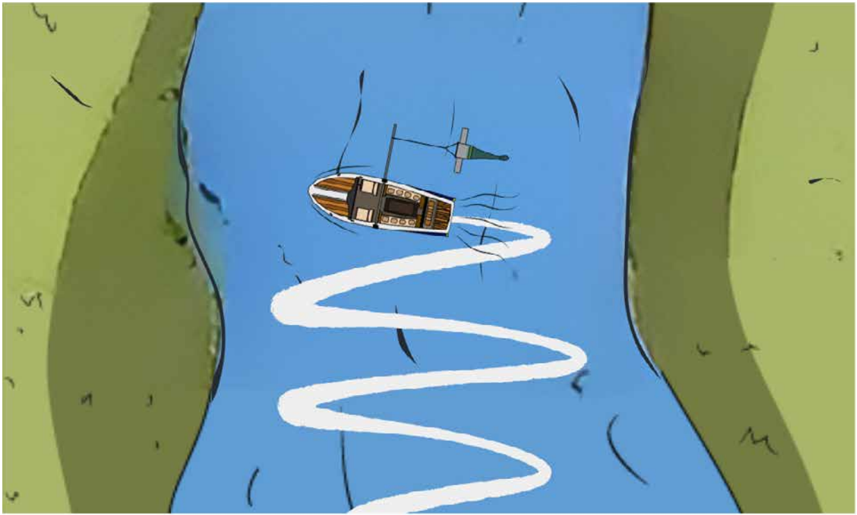
Figure 6: Zig-zag towing patterns are recommended to collect floating mesolitter in narrow channels.
