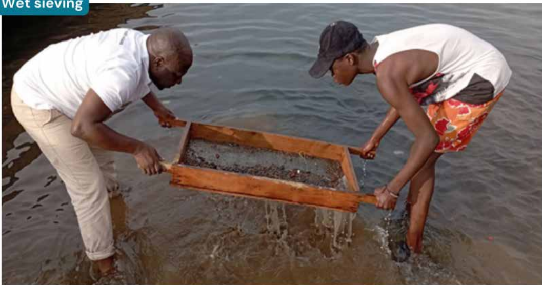
Figure 9: Dry sieving is done by adding sand to a sieve and shaking it (top), while wet sieving involves washing water over the sieve or dipping it on the water surface (bottom). Wet sieving has a greater environmental impact and is not recommended for use on the dry sand.
