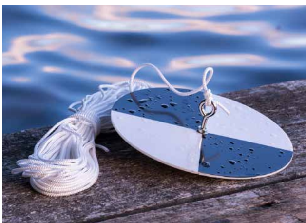
Figure 5: A Secchi disc, used to measure water transparency, can be made with cheap materials.
