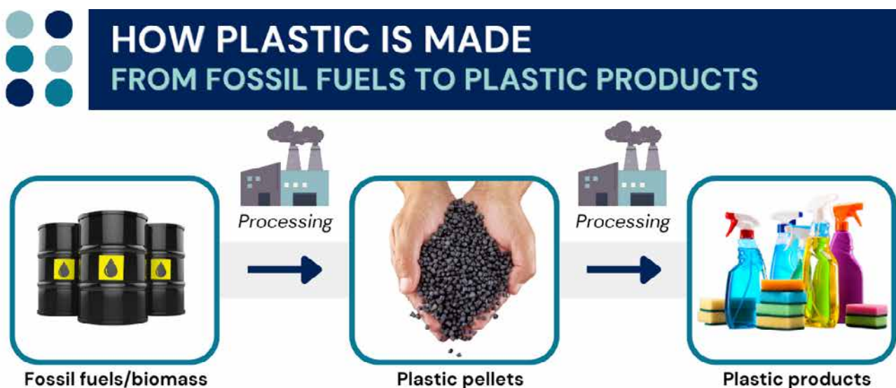
Figure 6: Plastic products are derived from either fossil fuels (crude oil, coal or natural gas), or from biomass (renewable resources such as sugarcane, corn or wood chips).
