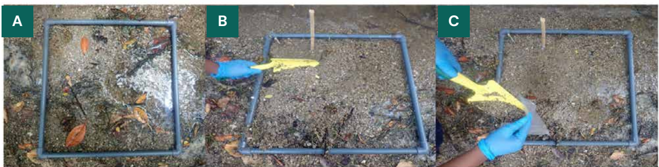
Figure 7: Sample collection for mesolitter using 0.5 m x 0.5 m quadrats. A marked stick is used as a ruler to indicate depth.
