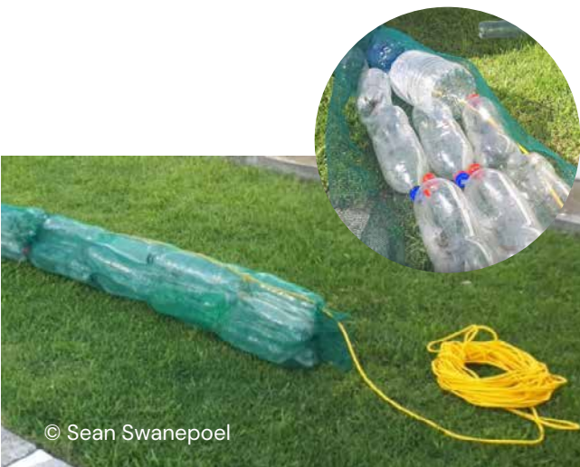
Figure 5: A plastic bottle boom uses empty plastic bottles as floats.
