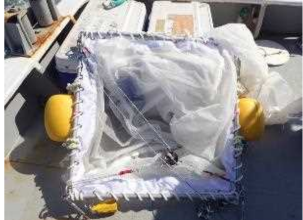
Neuston net with flow meter
