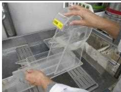
Use of Folsom splitter Splitter is moved back and forth to mix thoroughly, then the sample is divided.
