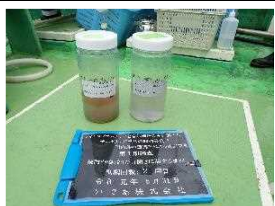
Fig.2-8. Plastic particles collected using nets with mesh openings of 0.35 mm and 0.10 mm at the same time in the same area (in CMSM2019).
