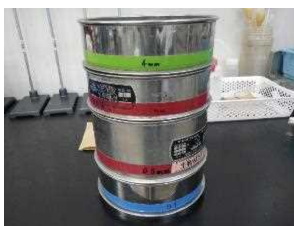
Multi-staged sieve with various mesh openings
