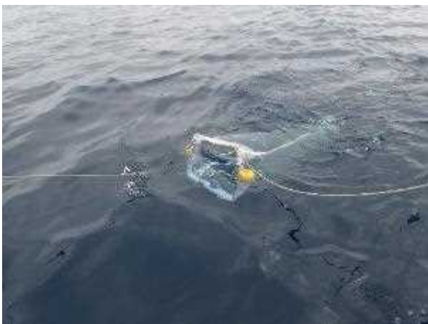
Fig.2-15. Adjustment of immersion depth of the Neuston net by attaching appropriate floats.
