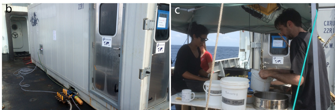
Figure 12. Typical cold filtered seawater (CFSW) setup on ABYSSLINE cruises. (a) Diagram showing the location of a constant temperature (CT) van on the back deck, with inflow of seawater from the ships pump (typically not filtered and at surface temperature of ~28 °C) into a filter, then a series of water containers in the cold room, then via controlled hoses back out of the van onto a sieving table (b,c). A system like this can store about 1000 litres of CFSW and provide water to sort 2–3 box cores over a 24 h period.
