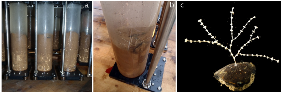
Figure 6. The multiple core (here a megacore type) is not normally a suitable sampling device for the CCZ as the macrofaunal abundances are too low. However, it can be used for opportunistic sampling from cores destined for other purposes—here a primnoid coral on a nodule has been sampled from a core destined for microbiology studies.
