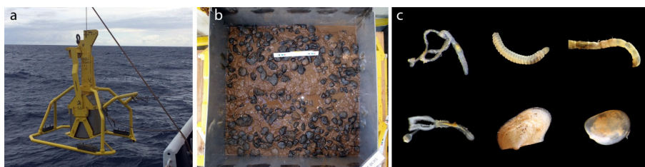
Figure 7. The Ocean Instruments BX-S50 MK-III Spade Core (BC) (a) is a highly effective sampling device for the CCZ, taking a large enough sample to be useful for macrofaunal studies, as well as a relatively undisturbed collection of polymetallic nodules and the sessile fauna that they support (b); Illustrated is a range of macrofaunal taxa typically less than 1 mm in size collected with box core on the recent ABYSSLINE program to the eastern CCZ (c).
