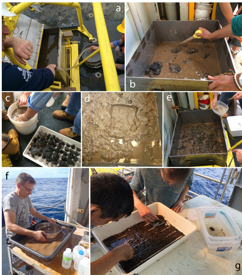
Figure 13. Processing mud samples from box core and EBS on deck. (a) Siphoning off the top-water from the box core onto 300 \mu\text{m} sieves; (b) Removing remaining surface water with a syringe/baster; (c) Picking large megafaunal and macrofaunal animals to a chilled CFSW container; (d) Picking nodules and rinsing them to remove mud prior to examination under microscope; (e) Cutting the box core (here a sub-sample for live-sorting for DNA taxonomy) prior to sieving; (f) Sieving mud from the box core in a submerged sieve under CFSW; (g) Picking the remaining heavy fraction of an EBS sample for small bivalves. These process are also illustrated in the Electronic Supplementary Information (Video).
