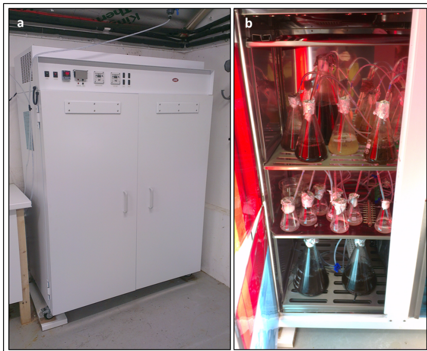
Figure 19: QUB Cultivation Cabinet. a: closed unit with temperature reading, timer switches and alarm (lights inset into doors); b: flasks in red (top two shelves) and blue light (bottom shelf) stage with individual air supply.
