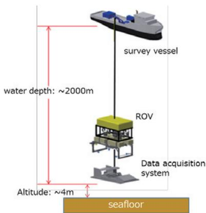
**Fig. 1** Schematic diagram of the magnetic measurement system using ROV
