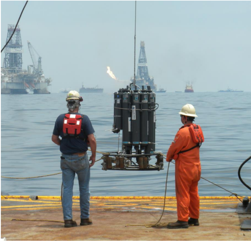
Figure 2. A CTD, typically used for temperature measurements as described here, is deployed following the Deepwater Horizon incident. Temperature profiles from such instruments are among the most common oceanographic observations conducted. Photo credit: Mark Bushnell
