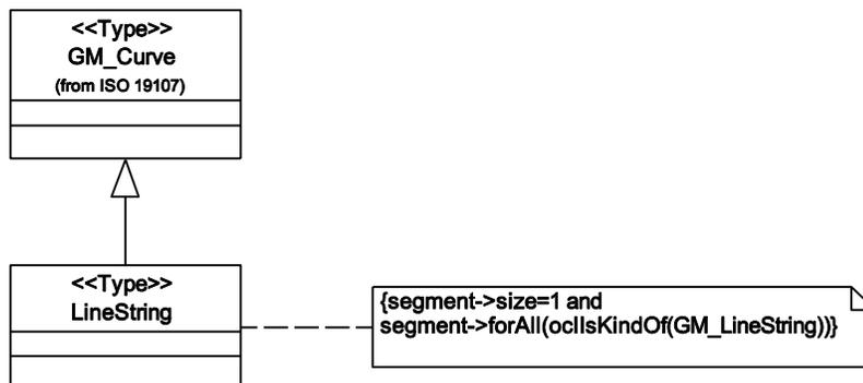
Figure 54 — GM\_Curve with a single GM\_LineString segment
