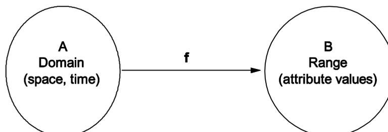
Figure 4 — Conceptual model of a coverage
