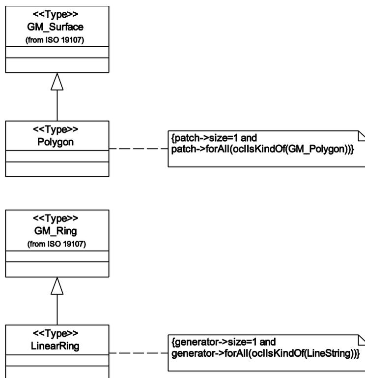
Figure 55 — A GM\_Surface with a single GM\_Polygon patch
