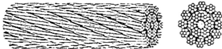
18 x 7 Non Rotating, Fiber Core
