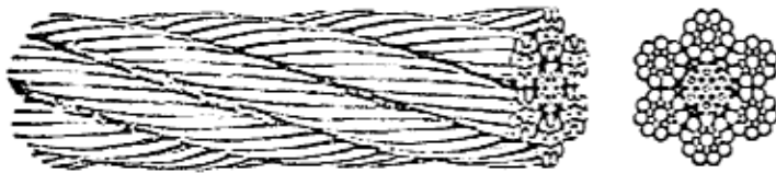
6 x 19 Searl Right Regular Lay, IWRC
